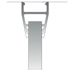
The continuous vertical profiles are drilled into the head rail to ensure optimum stability.
